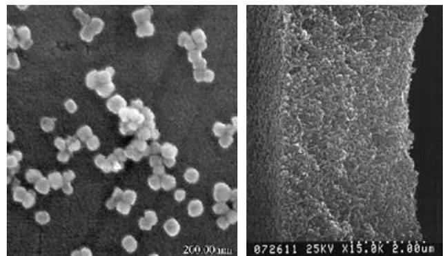
Figure 1. SEM image of TPL's ceramic nanoparticles (left) used in preparing the ceramic-polymer dielectric (right)
