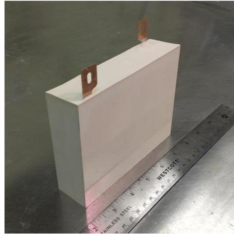
Figure 9. Photograph of scaled composite capacitor at 85 nF
