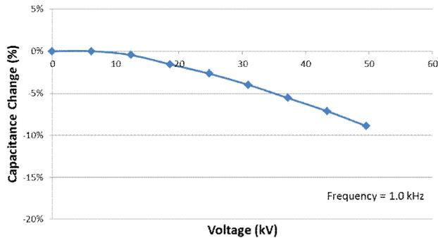
Figure 4. Capacitance change with voltage from 0 to 50 kV
