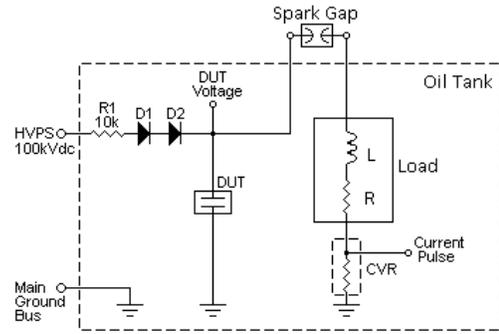
Figure 5. 100 kV RLC circuit used for capacitor life testing
