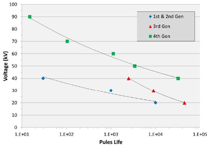
Figure 7. Discharge life testing results with power law curve fits, illustrate increased voltage and pulse life with continued capacitor development
