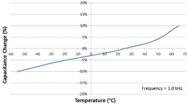
Figure 3. Capacitance change with temperature, -55 to 65 °C
