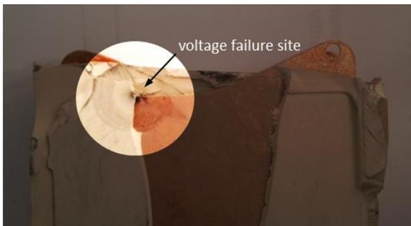
Figure 8. Dielectric breakdown of capacitor at electrode edge associated with electric field enhancement
