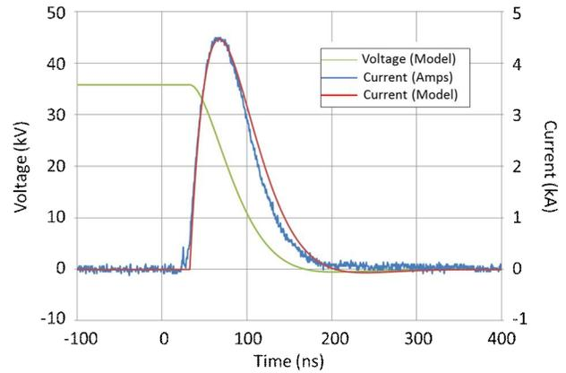
Figure 6. Discharge voltage and current measured on a 4<sup>th</sup> generation 9.6 nF capacitor into a 110 nH, 5.45  $\Omega$  load
