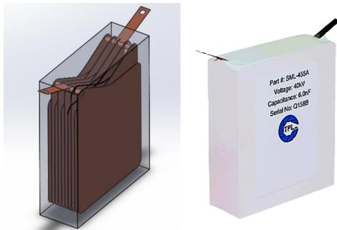
Figure 2. Schematic and photograph of the multi-layer, composite dielectric capacitors, left and right respectively
