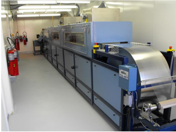
Figure 6: Pilot-scale solvent-cast film fabrication line, oven exit area
