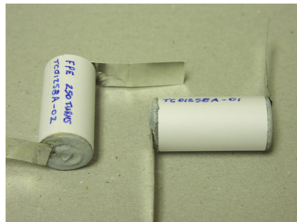
Figure 9: Wound and terminated FPE nanocomposite capacitor sections
